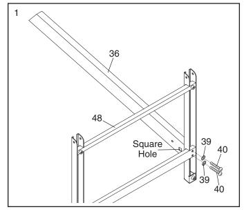
2. Orient the Left Upright (31) as shown, and attach it to the Base (48) with two Upright Bolts (40) and two Upright Star Washers (39); do not tighten the Upright Bolts yet.
